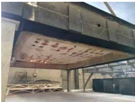
Figure 3. The underside of test assembly after fire testing.
