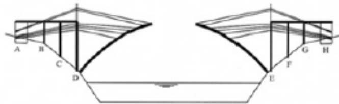
(b) Erection of Segments No. 6 to 11 and 18 to 23
