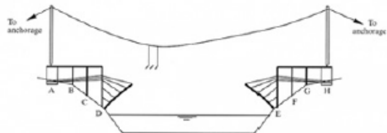
(a) Erection of Segments No. 1 to 5 and 24 to 28
