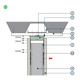
Deflection head parallel to floor profile for 15mm downward movement and up to 60 minutes fire resistance <sup>1</sup>
