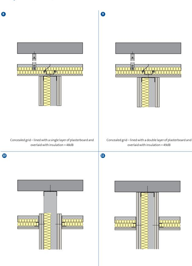
Concealed grid lined with a double layer of plasterboard within each room and overlaid with insulation = 56dB Partition lining continued to the soffit enabling the full potential of the partition to be achieved = 58dB
