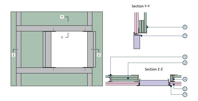
Opening between studs. Example shows 60mm stud
