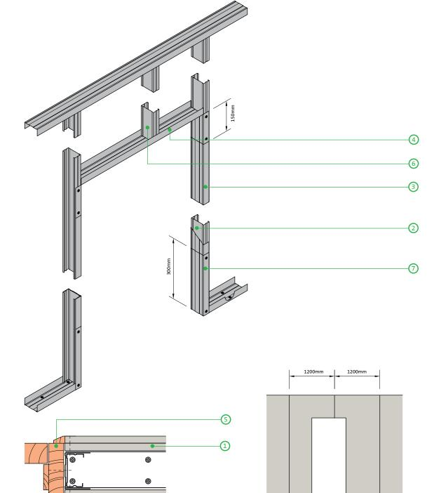
Door frame (maximum 1200mm width) to satisfy BS 5234: Parts 1 & 2: 1992 - Heavy and Severe Duty (up to 60kg door)
