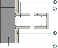
Junction with masonry and stop end
