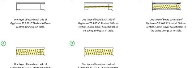
Gypframe 70 S 60 'C' Studs at 600mm centres. 80mm Isover Modular Roll in the cavity. Linings as in table.
