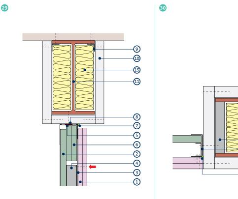
Beam encasement and partition junction for partitions to satisfy BS 5234: Parts 1 & 2: 1992 Heavy and Severe Duty Rating Column encasement and partition junction for partitions up to 120 minutes fire resistance and *BS 5234 Parts 1 & 2: 1992* Heavy and Severe Duty Rating
