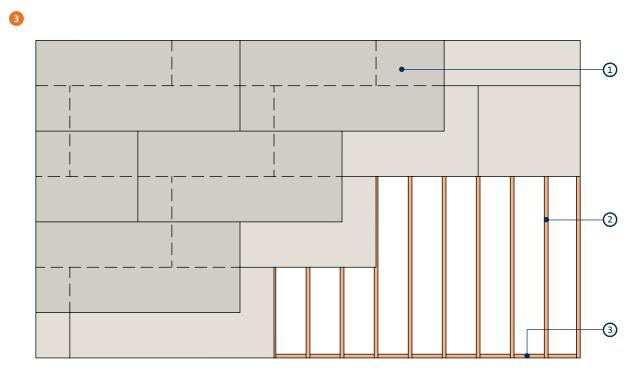
Reflected ceiling plan double layer - 12.5mm plasterboard with joists at maximum 450mm centres (noggings may be required to support long edges of board of outer layer if fire-rated)
