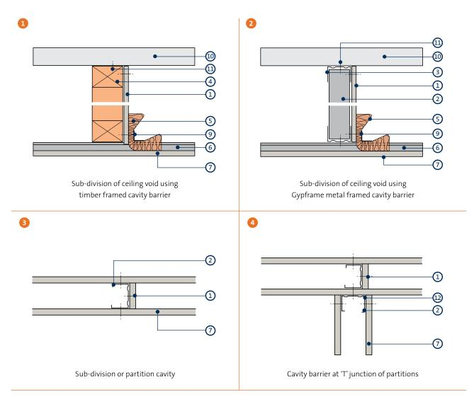
1 Gyproc plasterboard or Glasroc F specialist board forming cavity fire barrier
