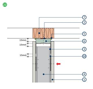
Deflection head perpendicular to floor profile for 15mm downward movement and up to 60 minutes fire resistance
