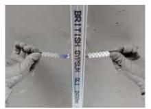
The protruding legs of each bracket are bent to sit back from the channel face. Gypframe GL1 Lining Channel sections are extended using Gypframe GL3 Channel Connectors.
