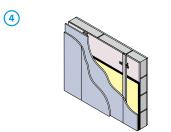
Solid block wall (100mm), of density 1700 kg/m<sup>3</sup> with 13mm plaster each side. Gypframe GL1 Lining Channel framework fixed to one side to give 35mm cavity. Cavity filled with 25mm Isover Acoustic Roll. Linings as in table.
