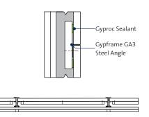
Horizontal board joints are fire stopped using Gypframe GA3 Angle and strips of Gyproc CoreBoard from the non-shaft side.
