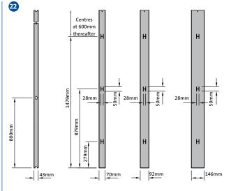
Gypframe studs service push-out details – Gypframe AcouStuds
