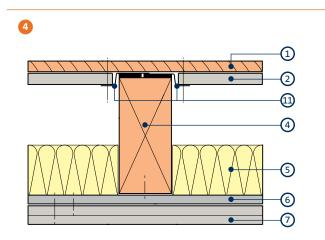
Section through floor - joist width over 75mm
