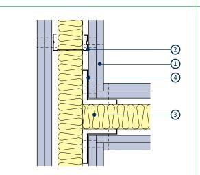
'T' junction to optimise acoustic performance and reduce flanking transmission
