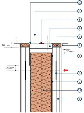
Deflection head for 15mm downward movement up to 240 minutes fire resistance
