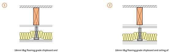
18mm t&g flooring grade chipboard and ceiling of Gyproc Plank and 12.5mm Gyproc WallBoard to simulate a wood lath and plaster ceiling<sup>2</sup>. **Gyplyner** ceiling<sup>1</sup> suspended with Gypframe GL1 Lining Channels at 450mm maximum centres to give a minimum cavity of 50mm to a maximum of 145mm. 50mm Isover Acoustic Roll in the cavity. Ceiling linings as in table. 100% loadbearing ratio.
