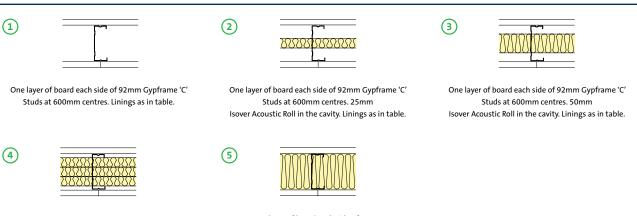
One layer of board each side of 92mm Gypframe 'C' Studs at 600mm centres. 3 x 25mm Isover Acoustic Roll in the cavity. Linings as in table. One layer of board each side of 92mm Gypframe 'C' Studs at 600mm centres. 100mm Isover Modular Roll in the cavity. Linings as in table.
