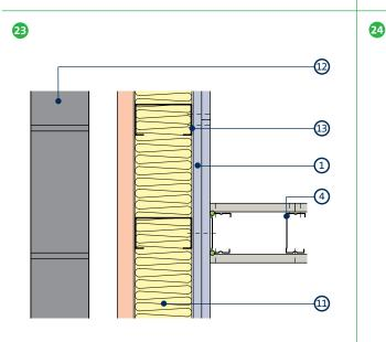
Junction with external wall Acoustic principles only. Fire performance of structural metal wall by others
