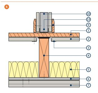
Non-loadbearing partition sited over joists
