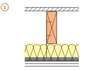
21mm t&g flooring over 38mm x 195mm (minimum) timber joists at 600mm (maximum) centres. **Gyplyner** ceiling fixed to underside of joists with Gypframe GL1 Lining Channels at 450mm maximum centres. 100mm Isover Spacesaver Ready-Cut in the cavity. Ceiling linings as in table. 100% loadbearing ratio.
