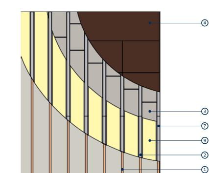
Cut-away floor plan (Chipboard flooring)
