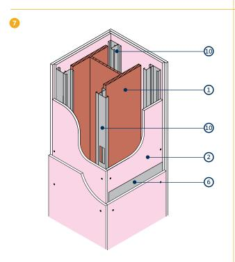
Boxing out for columns up to 600mm wide using GypLyner IWL
