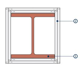
Four-sided column encasement for up to 120 minutes fire protection - double layer
