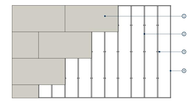
Reflected ceiling plan for flat soffit - single layer 15mm Gyproc plasterboard with channels at 600mm maximum centres, 12.5mm Gyproc plasterboard with channels at 450mm maximum centres, Gyptone board with channels at 600mm maximum centres or Rigitone board at 330mm maximum centres
