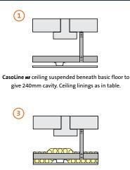
CasoLine we ceiling suspended beneath basic floor to give 240mm cavity, with 100mm Isover Spacesaver Ready-Cut in cavity. Ceiling linings as in table.
