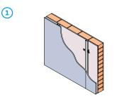
Solid brick wall (103mm) of density 1700 kg/m<sup>3</sup> with 13mm plaster each side and Gypframe GL1 Lining Channel framework fixed to **one side** to give 35mm cavity. Lining as in table.
