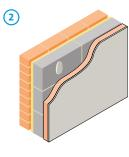
103mm brick skin, minimum 50mm clear cavity and 100mm block inner leaf. Linings as in table.
