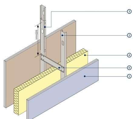
Splicing and solid bracing
