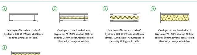
One layer of board each side of Gypframe 70 I 50 'I' Studs at 600mm centres. 75mm Isover Acoustic Slab in the cavity. Linings as in table.
