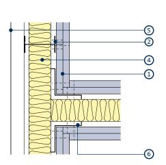
Partition junction Partition junction to optimise acoustic performance and reduce flanking transmission 7 8 5 8 4 2 1 ]/[ 0 Gyproc control joint - single board Gyproc control joint - double board
