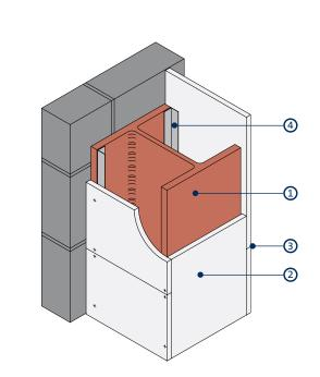
Four-sided column encasement for up to 120 minutes fire protection
