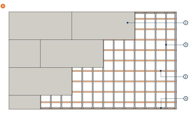
Reflected ceiling plan single layer - 12.5mm plasterboard with Gypframe RB1 Bars at maximum 450mm centres
