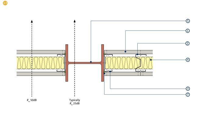
Exposed / painted steel column No fire protection to steel, Acoustic baseline only
