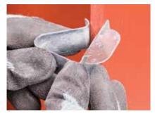
Four-sided protection to steel columns, Gypframe GL10 GypLyner Steel Framing Clips are friction-fitted onto the column / beam flanges at 800mm centres.
