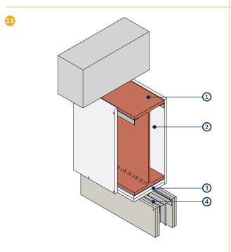
Beam encasement and partition junction for partitions up to 60 minutes fire resistance and *BS 5234* Light and Medium Duty
