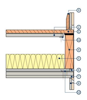
Perimeter junction - inner leaf of external wall exceeds mass of 365kg/m<sup>2</sup>
