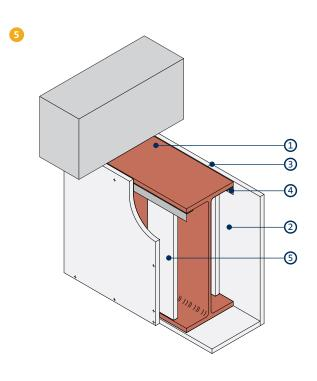
Three-sided beam encasement incorporating steel angles for up to 120 minutes fire protection
