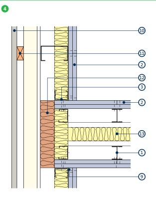
Junction with external wall when acoustic performance is a key consideration - Helps reduce flanking transmission
