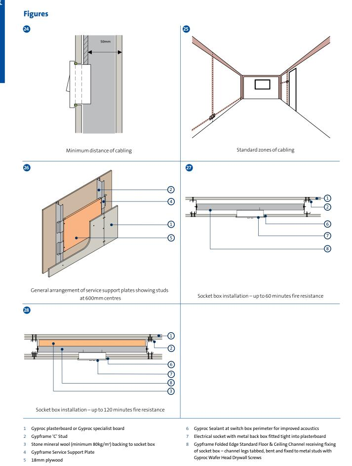
**NB** If Gypframe Service Support Plates are being installed and not immediately boarded, secure plates with a Gyproc Wafer Head Drywall Screw or Gyproc Wafer Head Jack-Point Screw.
