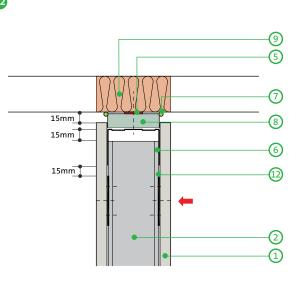
Deflection head parallel to floor profile for 15mm downward movement and up to 60 minutes fire resistance <sup>1</sup> Deflection head perpendicular to floor profile for 15mm downward movement and up to 60 minutes fire resistance
