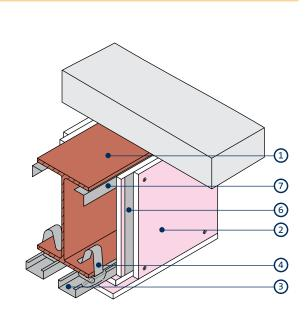
Three-sided beam encasement - double layer
