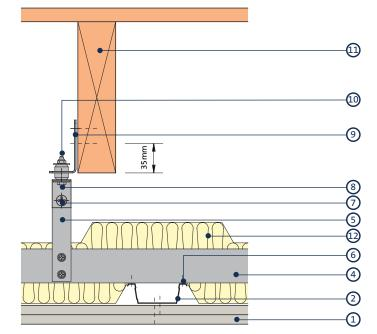
Suspension from timber joist using Gypframe Acoustic Hangers
