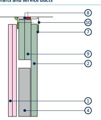
Head (sealed structure). Example shows 60mm stud<sup>3</sup>
