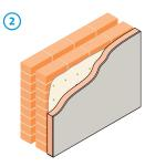
103mm brick skin, 50mm clear cavity and 103mm brick inner leaf with 13mm plaster. Linings as in table.
