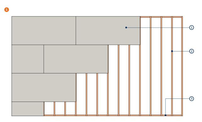
Reflected ceiling plan - single layer. 12.5mm plasterboard with joists at maximum 450mm centres (or 15mm plasterboard with joists at maximum 600mm centres)
