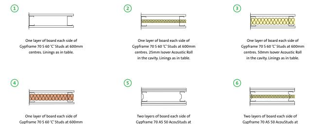
Gypframe 70 AS 50 AcouStuds at 600mm centres. 25mm Isover Acoustic Roll in the cavity. Linings as in table.
