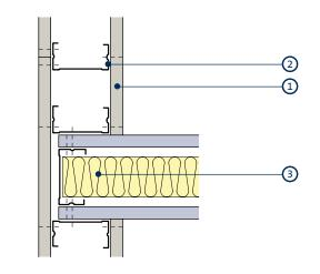
'T' Junction when partition with higher acoustic performance abuts a partition with lower acoustic performance. Acoustic principles only - detail may not be suitable for all solutions
