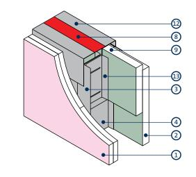
Head incorporating Gypframe G108 Retaining Clip (92mm)
