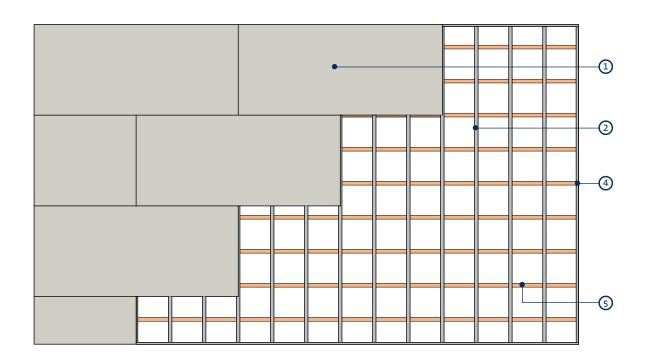
Reflected ceiling plan for timber joist floor - single layer 15mm Gyproc plasterboard with channels at 600mm maximum centres, 12.5mm Gyproc plasterboard with channels at 450mm maximum centres, Gyptone board with channels at 600mm maximum centres or Rigitone board at 330mm maximum centres
