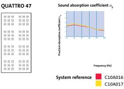
Gyptone QUATTRO 47 (plenum depth 400mm) Gyptone QUATTRO 47 (plenum depth 400mm plus 50mm Isover Roll)
