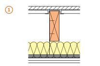
GypFloor SILENT comprising minimum 21mm t&g softwood floor boarding with Gyproc Plank on Gypframe SIF Floor Channels. GypLyner ceiling suspended with Gypframe GL1 Lining Channels at 450mm maximum centres. 100mm Isover Spacesaver Ready-Cut in the cavity. Ceiling linings as in table. 100% loadbearing ratio.
