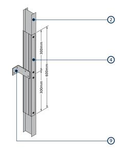
Gypframe 'I' Stud / splicing and bracing
