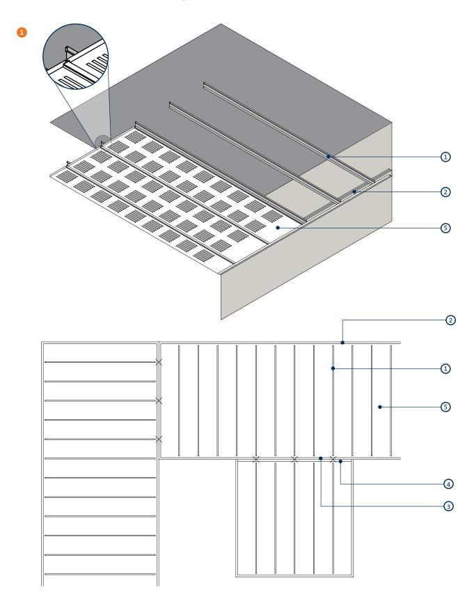
CasoLine дикк-юск Corridor System 15mm exposed metal grid fixing system for Gyptone Plank with edge E15/A
