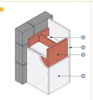
Three-sided column encasement incorporating Glasroc F FIRECASE soldiers for up to 90 minutes fire protection Three-sided column encasement incorporating steel angles for up to 120 minutes fire protection
