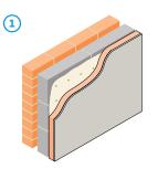
103mm brick skin, 50mm clear cavity and 100mm block with 13mm plaster. Linings as in table.
