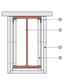
Three-sided beam encasement incorporating steel angles for up to 120 minutes fire protection - double layer
