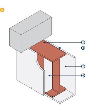
Three-sided beam encasement incorporating Glasroc F FIRECASE soldiers for up to 90 minutes fire protection
