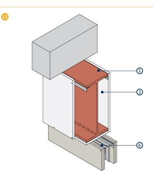
Beam encasement and partition junction for partitions up to 120 minutes fire resistance and *BS 5234* Heavy and Severe Duty
