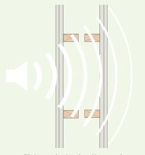
In an unfilled cavity, the plasterboard linings and cavity alone provide the sound insulation which can result in poor performance and a hollow sounding construction.
