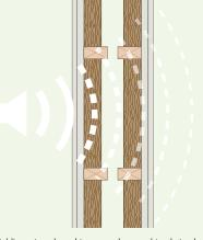
Adding mineral wool improves the sound insulation by absorbing reverberant sound within the cavity therefore reducing the amount of sound energy transferred from one side of the construction to the other.
