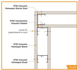
► See Construction Details Drawings for further guidance on arrangement and fixing.
