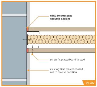
PT-CS-506P-Acoustic rated T-junctions, double layer
