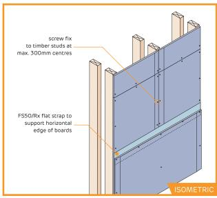
► GTEC Timber Single Stud partition system is suitable for single, double and multiple layer boarding.
