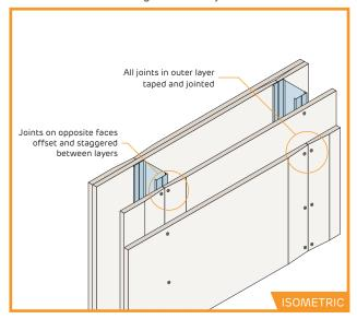
PT-CS-204M-Horizontal joint reinforcement, double layer
