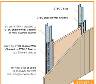
PT-CS-803M-Timber support for extreme-weight fixings
