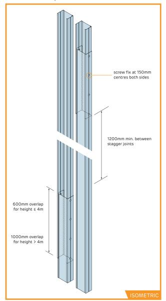
PT-CT-105M-V-brace fixing and extensions
