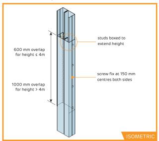
➤ Select compatible size (e.g. 70mm stud and 72mm track) GTEC Resilient Acoustic Stud, GTEC C Stud and GTEC U Track framing elements to suit system performance.
