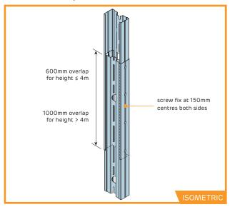
➤ Select compatible size (e.g. 70mm stud and 72mm track) GTEC Acoustic Stud, GTEC C Stud and GTEC U Track framing elements to suit system performance.
