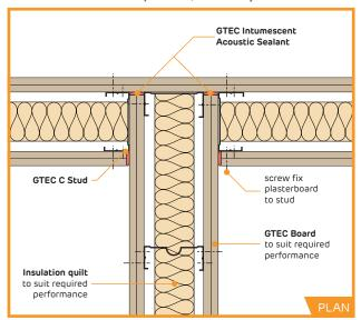
► GTEC C Studs to be used at corners and junctions to provide flat web for fixing.
