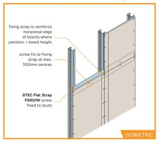
PT-AH-203M-Board fixing - single layer
