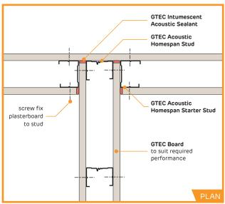
► GTEC Acoustic Homespan Starter Studs to be used at corners and junctions to provide flat web for fixing.
