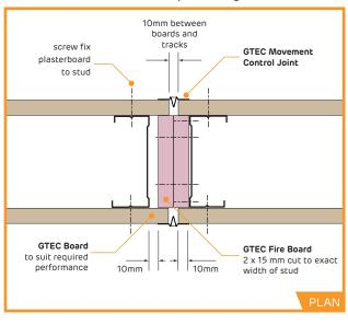
PT-CS-302P-Movement control joint - double boarded
