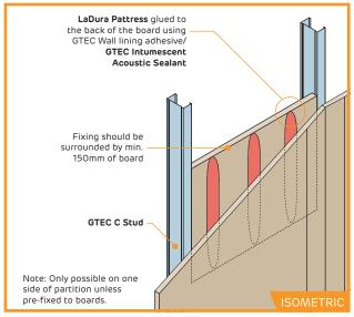
PT-CS-805M-LaDura channel pattress for heavy-weight fixings
