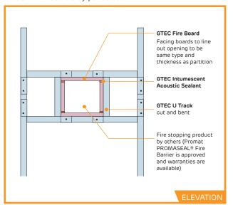
PT-CS-703M-Cable tray penetration at soffit
