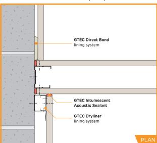
PT-CS-514P-T-Junction of Twin into Single Frame
