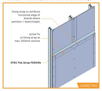
► GTEC Resilient Acoustic Stud partition system is tested with double boarding only; refer to performance tables on p29-36.
