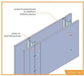
► GTEC Acoustic Stud partition system is suitable for single, double and multiple layer boarding.
