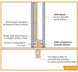
PT-TS-104S-Base Detail (Non-Load Bearing)
