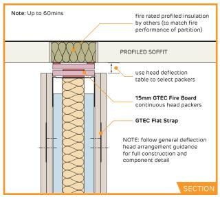
PT-CS-604S-Def. Head – perpendicular to simple profile
