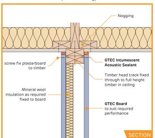
PT-TS-102S-Head Detail (Non-Load Bearing)
