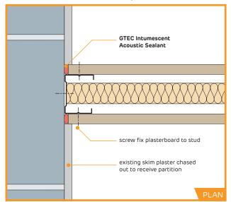
PT-CS-513P-T-Junction of Single into Twin Frame
